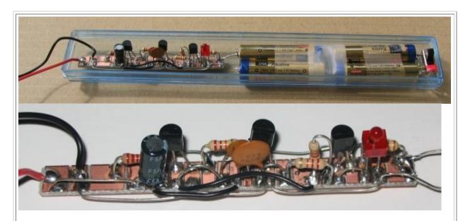
The transmitter is built on a small length of PC board, cut into lands with a file. The photo clearly shows how all the components are mounted and how the board is fitted into a toothbrush holder. The flashing LED shows the unit is ON and serves to control the beep-beep of the circuit. The flashing LED is not an ordinary LED.
