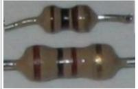
The 1/10th watt resistors used in this circuit, compared with 0.25watt resistors.
