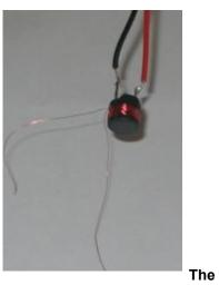
10mH choke with 150 turns for the secondary
