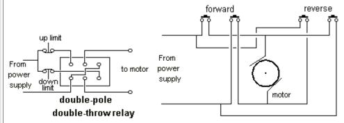
The way the dpdt relay circuit (above) works is this:
