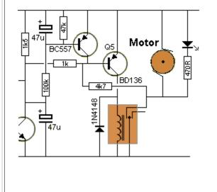
A normal relay can be activated by a short tone and de-activated by a long tone as shown via the circuit on the left. This circuit can be found in **"27MHz Links"** Page 2.
