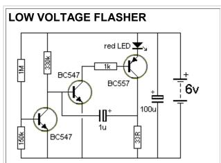
This circuit flashes when the voltage drops to 4v. The voltage "set-point" can be adjusted by changing the 150k on the base of the first transistor.
