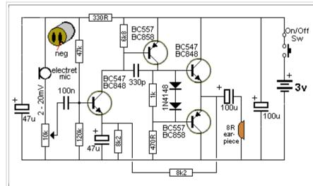
emitter of the first transistor and 0v rail and the 470R resistor. The 8k2 across the 47u sets the emitter voltage on the BC 547 and this turns it on. The collector is directly connected to the base of a BC 557, called the driver transistor. Both these transistors are now turned on and the output of the BC 557 causes current to flow through the 1k and 470R resistors so that the voltage developed
