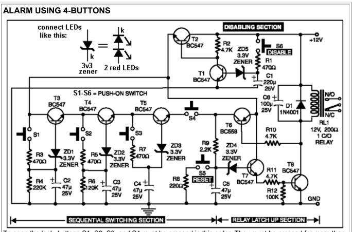
To open the lock, buttons S1, S2, S3, and S4 must be pressed in this order. They must be pressed for more than 0.7 seconds and less than 1.3 seconds.
