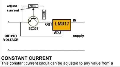
few milliamp to about 500mA - this is the limit of the BC337 transistor.
