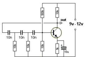
This circuit produces a sinewave very nearly equal to rail voltage.
