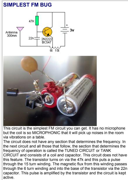
The frequency is determined by the 6 turn coil. By moving the turns together, the frequency will decrease. The circuit transmits at 90MHz. It has a very poor range and consumes 16mA. The coil is wound on a 3mm drill and uses 0.5mm wire.
