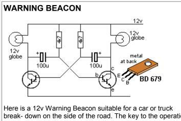
break- down on the side of the road. The key to the operation of the circuit is the high gain of the Darlington transistors. The circuit must be kept "tight" (thick wires) to be sure it will oscillate.
