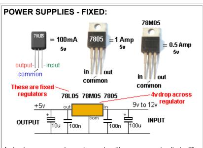
A simple power supply can be made with a component called a "3pin regulator or 3-terminal regulator" It will provide a very low ripple output (about 4mV to 10mV provided electrolytics are on the input and output.
