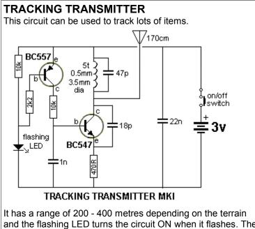
and the flashing LED turns the circuit ON when it flashes. The circuit consumes 5mA when producing a carrier (silence) and less than 1mA when off (background snow is detected).
