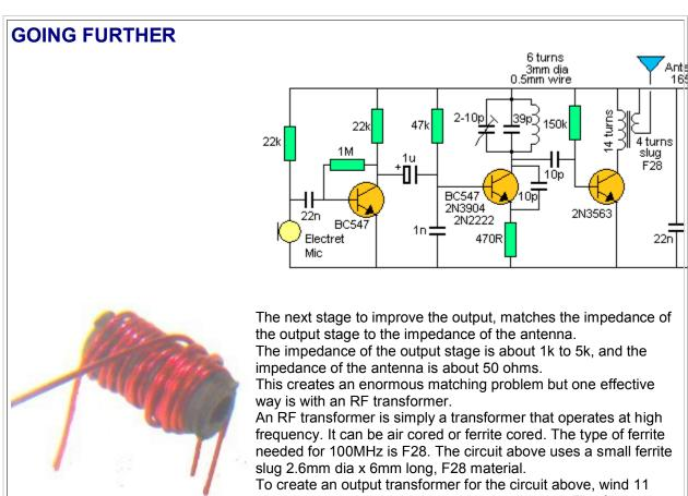
turns onto the slug and 4 turns over the 11 turns. The ferrite core will do two things. Firstly it will pass a high amount of energy from id secondly it will
