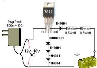
This is a very simple battery charger to keep a battery "nearly fully charged."
