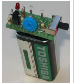
The regulator connected to a 9v battery
