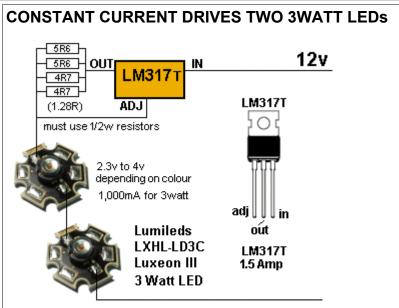
The value of the current-limiting resistor: Resistor(Ohms) = 1.25(V) /current(A)
