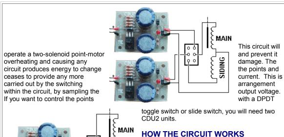
The circuit is supplied by 16v AC or DC and the diode on the input is used to rectify the voltage if AC is supplied. If nothing is connected to the output, the base of the BD679 is pulled high and the emitter follows. This is called an emitter-follower stage. The two 1,000u electrolytics charge and the indicator LED turns on. The circuit is now ready. When the Main or Siding switch is pressed, the
