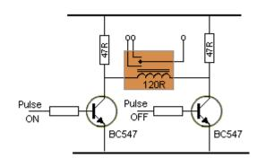
A single-coil latching relay normally needs a reverse-voltage to unlatch but the circuit at the left provides forward and reverse voltage by using 2 transistors in a very clever H-design.
