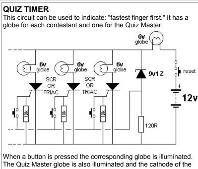
The Quiz Master globe is also illuminated and the cathode of the 9v1 zener sees approx mid-rail voltage. The zener comes out of conduction and no voltage appears across the 120R resistor. No other globes can be lit until the circuit is reset.
