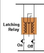
Latching Relays are expensive but a 5v Latching Relay is available from: <u>Excess Electronics</u> for \$1.00 as a surplus item. It has 2 coils and requires the circuit at the left. A 5v Latching Relay can be use on 12v as it is activated for a very short period of time.
