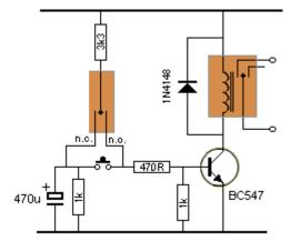
A double-pole (ordinary) relay and transistor can be connected to provide a toggle action.
