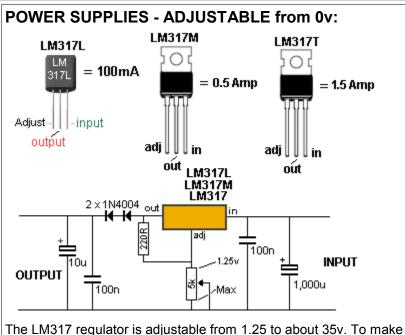
The LM317 regulator is adjustable from 1.25 to about 35v. To make the output 0v to 35v, two power diodes are placed as shown in the circuit. Approx 0.6v is dropped across each diode and this is where the 1.25v is "lost."
