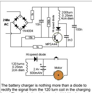
base. Thus the battery is in constant trickle charge as long as the hand unit is in the base. The battery pack is a pair of 600mAhr AA NiCd cells.
