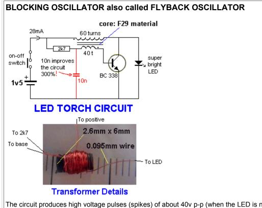
The circuit produces high voltage pulses (spikes) of about 40v p-p (when the LED is not connected), at a frequency of 200kHz. The super-bright LED on the output absorbs the pulses and uses the energy to produce illumination. The voltage across the LED will be about 3.6v
