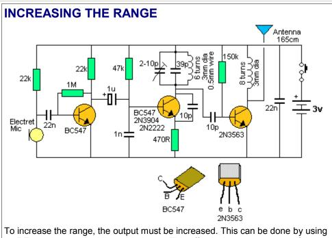
an RF transistor and adding an inductor. This effectively converts more of the current taken by the circuit (from the battery) into RF output. The output is classified as an untuned circuit. A BC547 transistor is not suitable in this location as it does not amplify successfully at 100MHz. It is best to use an RF transistor such as 2N3563.
