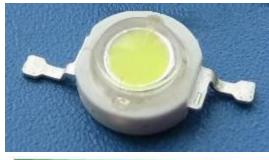
The circuit will not drive two LEDs in series - it runs out of voltage (and current) when the voltage across the load is 7v. It oscillates at approx 200kHz. Build both the 20 LED and 1 watt LED version and compare the brightness and effectiveness. The photo of the 1 watt LED on the left must be heatsinked to prevent the LED overheating. The photo on the circuit diagram shows the LED mounted on a heatsink and the connecting wires.
