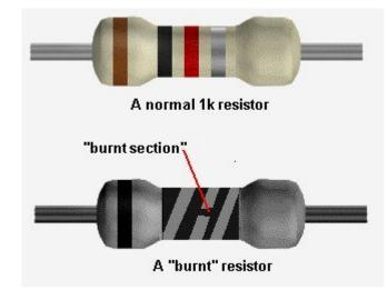
Clean the "spot" (burnt section of the spiral) very carefully and make sure you can get a good contact with the spiral and the tip of your probe. Measure from one lead of the resistor to the end of the damaged spiral. Then measure from the other lead to the other end of the spiral.
