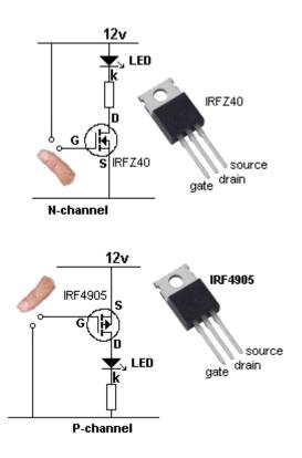
Touching the Gate will increase the voltage on the Gate and the MOSFET will turn on and illuminate the LED. Removing your finger will turn the LED off.
