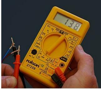
Measuring resistance of a heater (via the leads)
