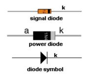
The best thing to do with a "suspect" diode is to replace it. This is because a diode has a number of characteristics that cannot be tested with simple equipment. Some diodes have a fast recovery for use in high frequency circuits. They conduct very quickly and turn off very quickly so the waveform is processed accurately and efficiently. If the diode is replaced with an ordinary diode, it will heat up as does not have the high-speed characteristic.
