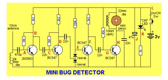
**Point A** - The first transistor is "self-biased" and will have 0.6v on the base. The antenna is connected to a 20 turn coil and you might think the coil will "short" the signals to earth.
