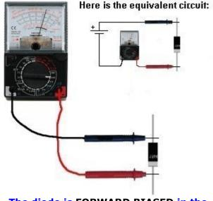
The diode is FORWARD BIASED in the diagram above and it conducts
