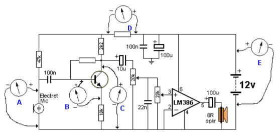
**MEASURING VOLTAGES IN A CIRCUIT**
