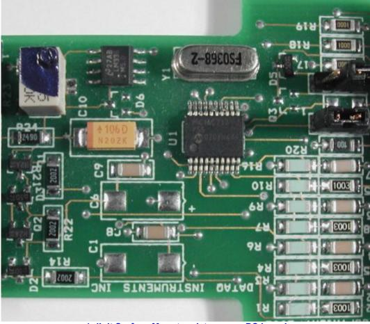
4-digit Surface Mount resistors on a PC board
