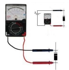
The diode is REVERSE BIASED in the diagram above and diodes not conduct.
