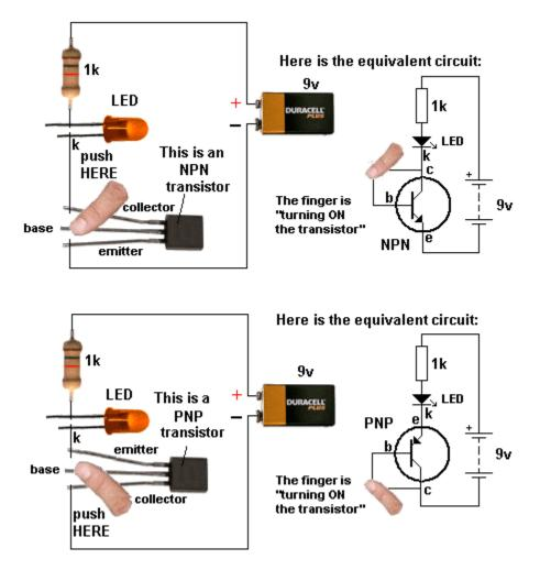
The leads of some transistors will need to be bent so the pins are in the same positions as shown in the diagrams. This helps you see how the transistor is being turned on. This works with NPN, PNP transistors and Darlington transistors.
