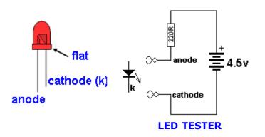
Connect the clips to a LED and it will illuminate in only one direction. The colour of the LED will determine the voltage across it. You can measure this voltage if you want to match two or more LEDs for identical operation.
