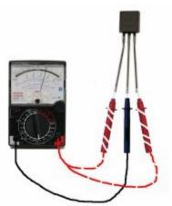
This is an NPN transistor The black probe is the BASE
