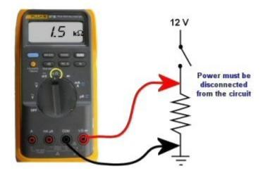
Measuring the resistance of a resistor
