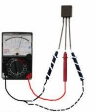
This is a PNP transistor The red probe is the BASE
