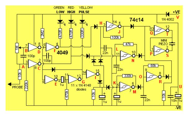
The voltage on a circuit (to be tested) is detected by the probe at **Point A** of the circuit above and the "tip" is classified as "reasonably high impedance" as it has a 220k resistor between the tip and 0v rail. The 1M reduces the impedance by about 20% but the inputs of the two inverters have no effect on the "tip" impedance as they are extremely high input-impedance devices.
