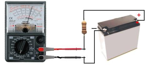
Measuring current through a resistor
