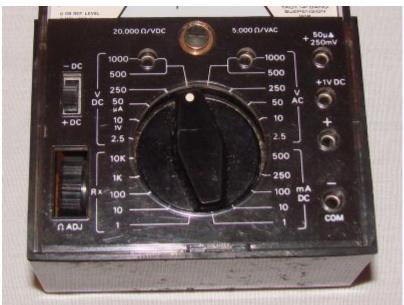
"Ohms Adjust" is also called "ZERO SET" The sensitivity of this meter is 20,000ohms/volt on the DC ranges and 5k/v on the AC ranges
