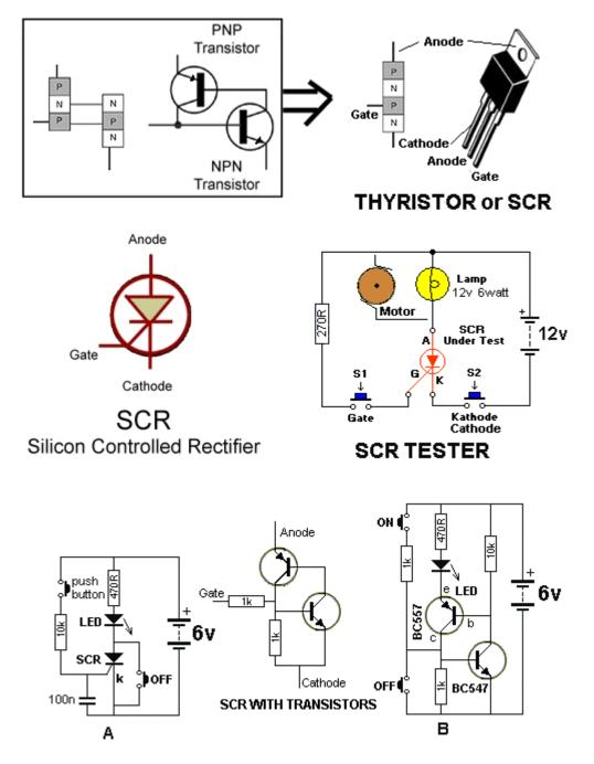
To understand how an SCR "latches" when the gate is provided with a small current, we can replace it with two transistors as shown in diagram B above. When the ON button is pressed, the BC547 transistor turns on. This turns ON the BC557 and it takes over from the action of the switch.
