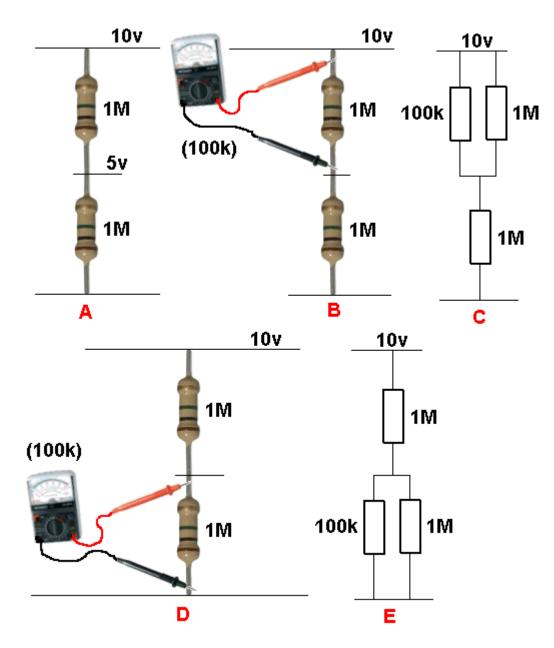
This introduces two new terms: <u>HIGH IMPEDANCE CIRCUIT</u> and "RESISTORS in <u>SERIES</u> and <u>PARALLEL</u>."
