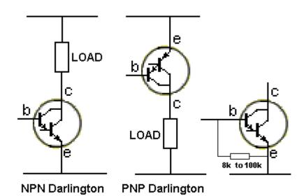
Darlington transistors are tested the same as an ordinary transistor and a multimeter will produce about the same deflection, even though you will be measuring across two junctions, (and a base-emitter resistor is present).
